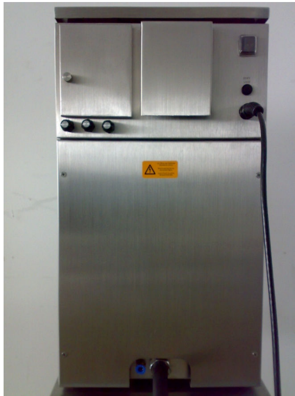
Fig. 6-6 External connection, Connection-Hub type (back view of cabinet)
