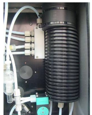
Fig. 3-1 Anti-explosion ripple cover
