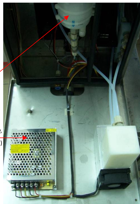
Fig. 8-4 condenser kit Incl. Air filter, Cooling kit with fan, Power supply, Magnetic valve
